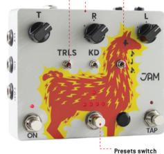
leftmost is a simple bypass. The center switch enables selection of the presets. It also enables selections from the four extreme modes—vibrato, tape-age, random, and pitch-shift—when used with the "alt" push-button just to the right of the footswitch. The rightmost footswitch is for controlling the tap tempo, but also engages the self-oscillation function when you press and hold.
